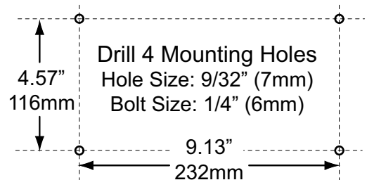
Figure 2: Drill Pattern and Hardware
