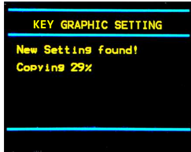
Figure 30. Downloading Graphics File to coder from USB Key
