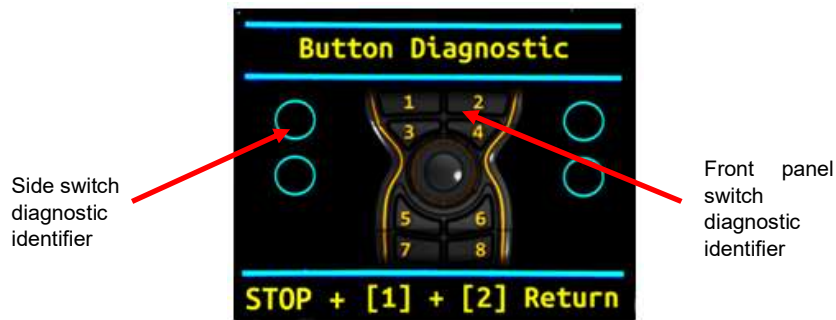
Figure 28. Button Diagnostic page on Transmitter
