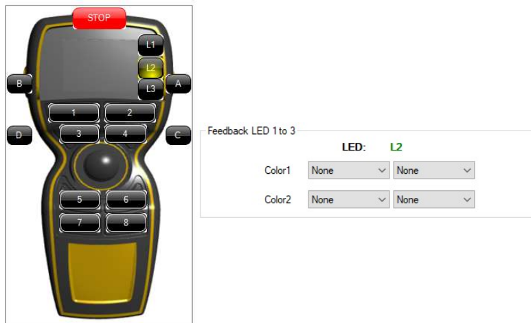
Figure 22. Setting the Sources for Feedback LED 2
